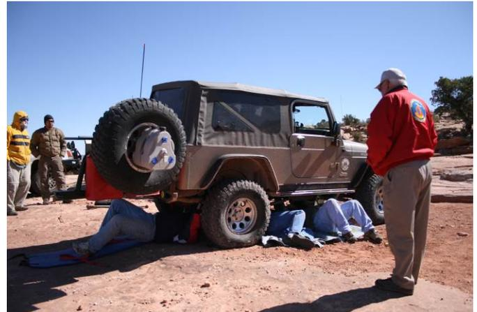
The whole Dirt Devil team jumped in. First we decided I could drive out with only one control arm. We removed the driver side rear upper control arm. I drove forward and got the pumpkin to rotate back down. Using the bolt out of the driver side control arm, we reinstalled the rear passenger side control arm. The Jeep was winched sideways to align the rear
